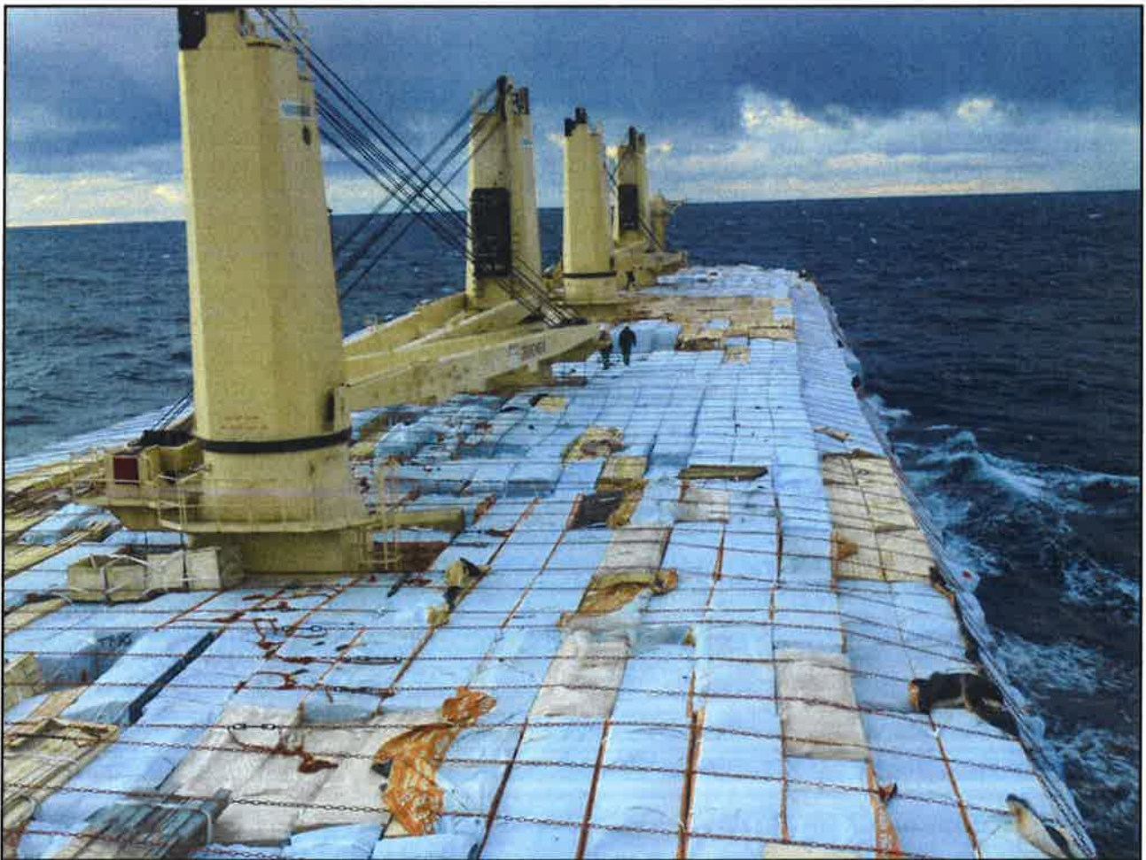
Figure 2: Graig Rotterdam at sea with timber deck cargo secured by top-over lashings
