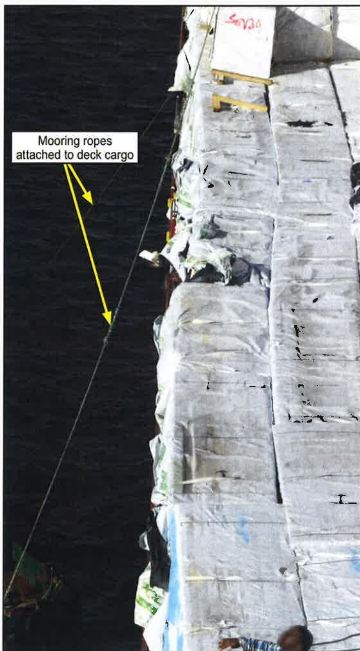
Figure 3: Cargo barges secured to deck cargo packages
